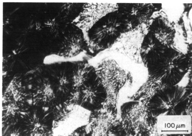
Figure 7 Optical micrograph (crossed polars) of deformed LDPE inclusion in iPP matrix
